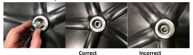
Step 10: Place a new bearing on the end of the hub
