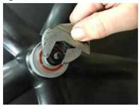
Step 13: Visually inspect to see that axle spacer is centered in bearings and then install end caps.
