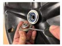
Step 4: Clean off the end caps and install the new seals (and new O rings in groove, if needed) as shown below. Make sure to press the new seals all the way down until they bottom out. \*NOTE: Some older generations of end caps may be slightly too large to fit the new seals. If this is the case, simple do not use the seals. The bearings themselves are sealed. Be careful not to rip the seals when installing.
