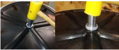
Step 7: Place a new bearing onto the end of the hub. Then, while holding the bearing, place the tool kit through the center of the hub and through the center of the bearing on the other side as shown below.
