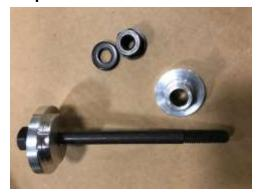
Step 6: Use the long pin in the tool kit to tap out the axle and bearing from one side of the hub. Flip the wheel over and use the pin to knock out the other
