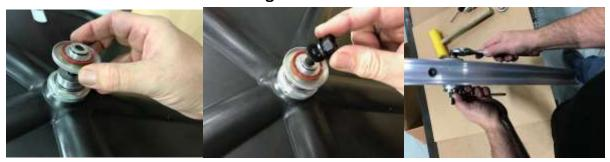
This first tightening operation pulls one bearing into place.
